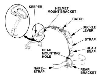
Figure 2-22. Installation of Helmet Mount.
